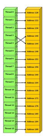
**Figure 6:** Left: Coalesced memory access. Right: Non-sequential non-coalesced memory access.
